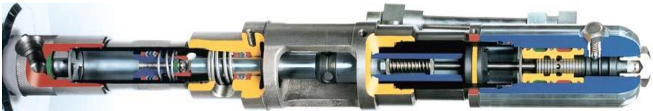
Cut-away Hydraulic Variable piston Pump
